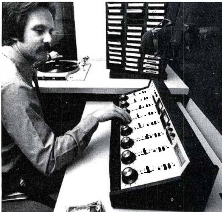
New Cetec Model 2003 8-mixer audio console.
